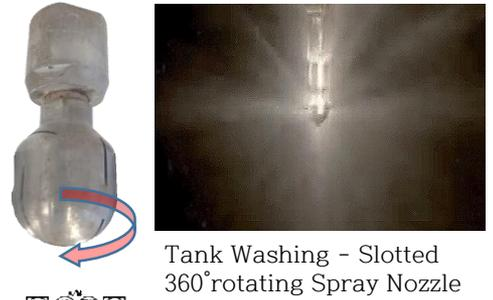
Tank Washing - Slotted 360° rotating Spray Nozzle
