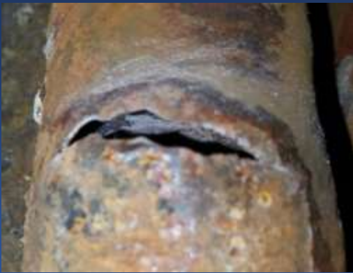
▷ Rupture of tube by local overheating
