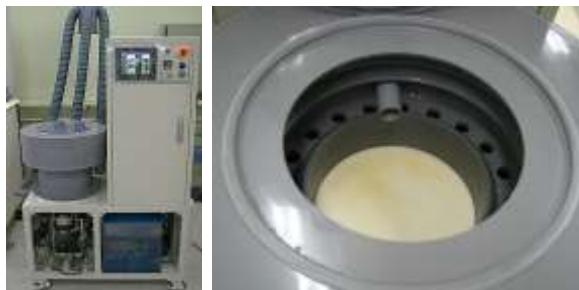
8inch proto(dip-spin) Thinning chamber Thinner(made in 2008)
