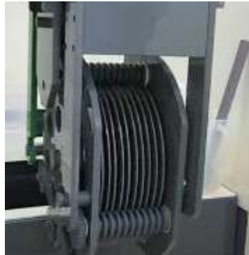
Wafer supported by ring frame is inserted into rotating barrel
