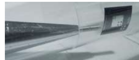
Bendable chip : 5*5mm , 6μm
