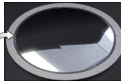
Mirror surface: damage relief and thinning
