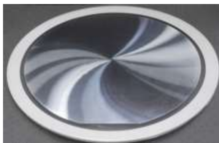
Grinded wafer : 2,000grit , THK: 200 µm
