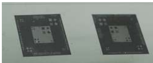
50 μm chip on protecting tape for thinning
