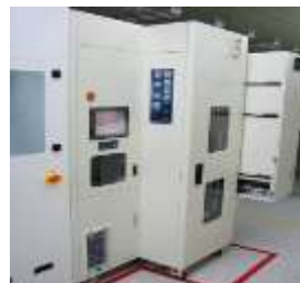
8inch wafer mass production equipment : 150 \mu m \rightarrow 50 \mu m , 16wph (made in 2007)
