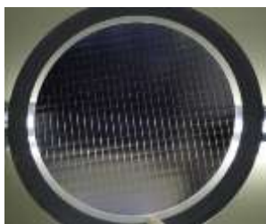
#12,000 grit ground 12 inch DBG Wafer use of #4800 dicing saw
