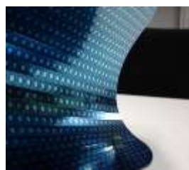
50 μm wafer ground by DBG
