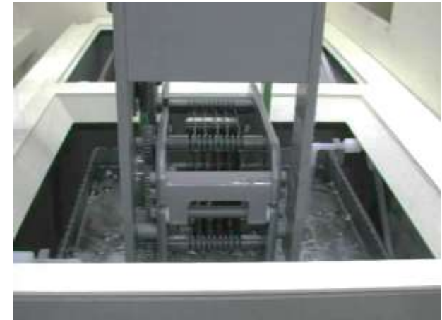
Barrel etcher for ultra thinning or damage relief
