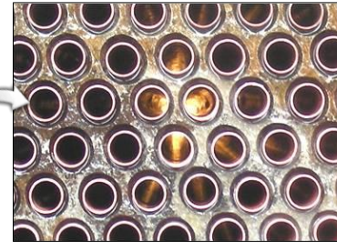
Carbon steel EX / Dip or Circulation 1~2 days / @25~40°C
