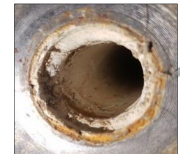
Cooling water piping / Dip or Circulation 2~4hr / @25~40°C
