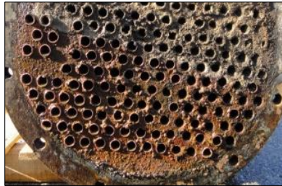
Carbon steel EX / Dip or Circulation 1~2 days / @25~40°C
