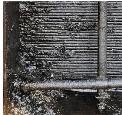
Hydrocarbon + silicate scale
