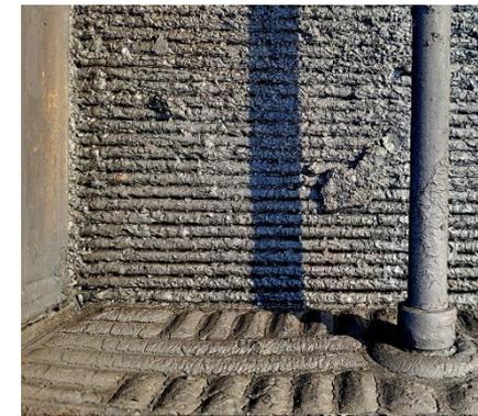
Hydrocarbon + sediments scale
