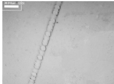
KOH 40% @80°C , 3μm etching (The fine wheel mark is expanded)
