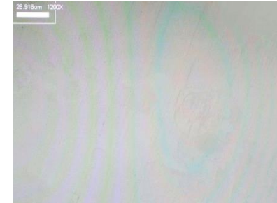
Slight etchant 25°C @120sec , 1μm etching (The wheel mark is reduced)
