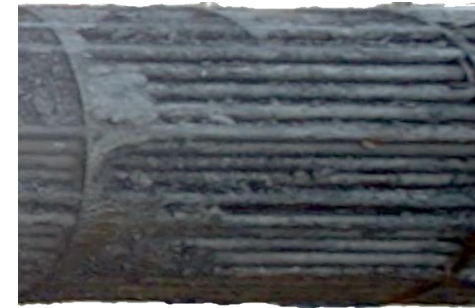
△ fouled heat exchanger
