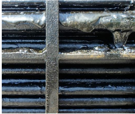
Heavy Hydrocarbon, Asphaltene, Tar / Dip 2~4hr / @80~90°C
