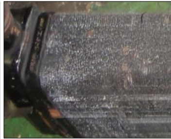
Aluminum Fin / Dip 10~30min / @35~50°C
