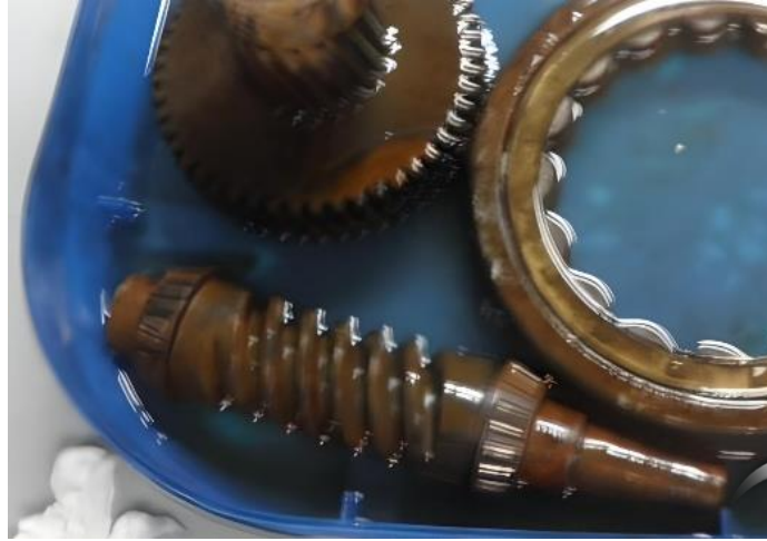
Grease + rusty bearing parts / Dip and/or ultra sonic cleaning 30~ 60min /@25~40°C
