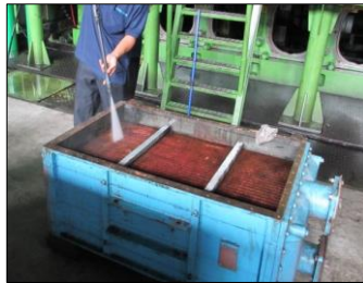
Copper fin Inter Cooler / Spray / @25~30°C
