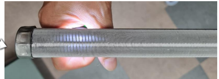
BOLL Cande Oil Filter / Dip & high pressure rinsing 60min /@100°C, boiling
