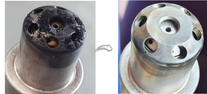
Oil Burner Nozzle / Dip & Boiling, U/S 30~60minhr / @100°C
