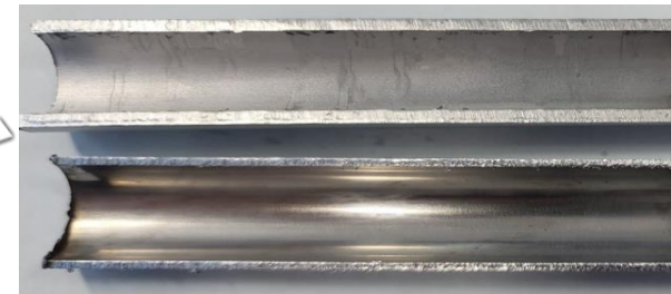
Drawing Oil / Dip & circulation 310~0min / @60~90°C
