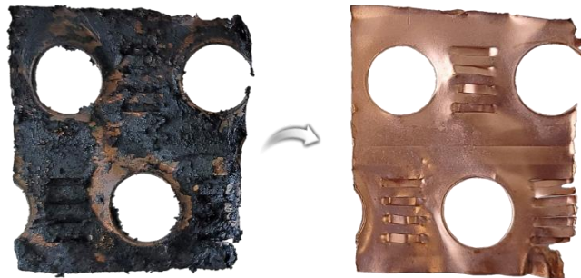
Carbonized organic matter by oil vapor on fin
