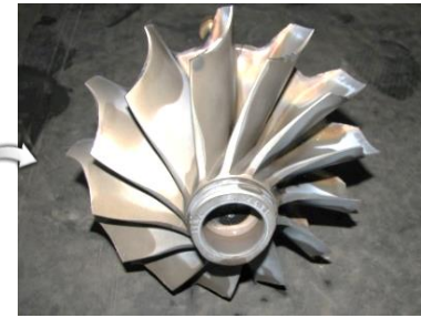
Aluminum alloy impeller / Dip 10~30min / @ 50~80°C
