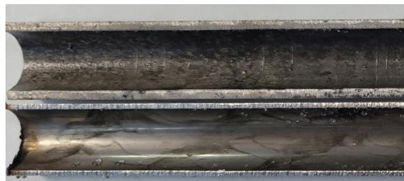
Stainless Steel(SUS-304/316) Seamless steel by Pilger Oil Drawing
