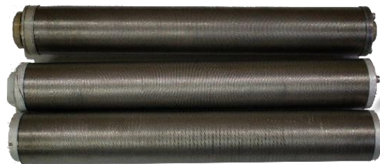
Notch Oil Filter / Dip & Ultra Sonic cleaning 30min @100°C, boiling
