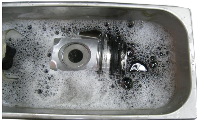
Engine Piston / Dip & Ultra Sonic cleaning 30min @90°C
