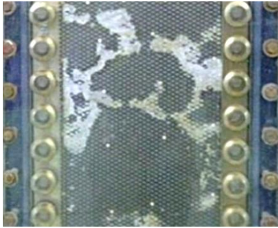
Chlorinator 전극 : before cleaning (power plant-Korea)
