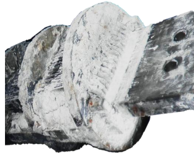
Chlorinator 전극 : before cleaning (power plant-Indonesia)
