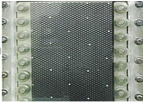
Chlorinator 전극 : After cleaning
