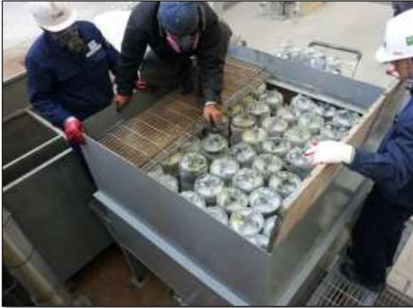
1. Insert the used filter in cleaning tank
