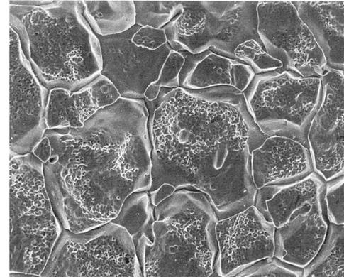
△ Grain boundaries are revealed by corrosion caused by mixed acid.
