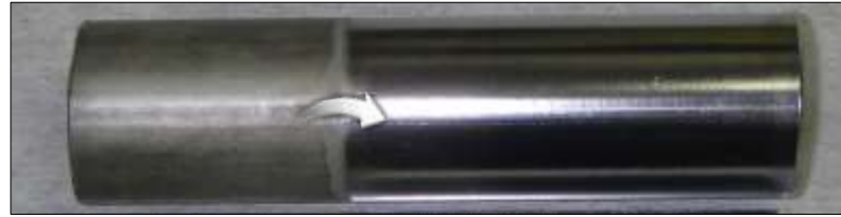
Chemical polishing of carbon steel pipe (SS41)
