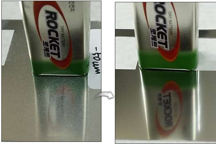
Invar sheet surface chemical polishing
