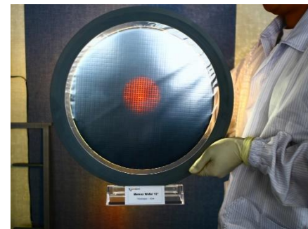
12inch 50 \mu\text{m} Memory wafer thinned down to 15 \mu\text{m}
