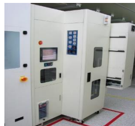
8inch wafer mass production equipment : 150um→50um , 16wph (made in 2007)
