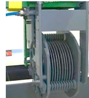
Barrel etcher for ultra thinning or damage relief
