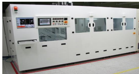
8inch wafer mass production equipment : 150um→50um , 16wph (made in 2007)
