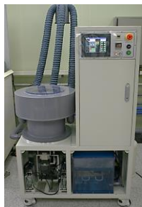
8inch proto(dip-spin) Thinning chamber Thinner(made in 2008)
