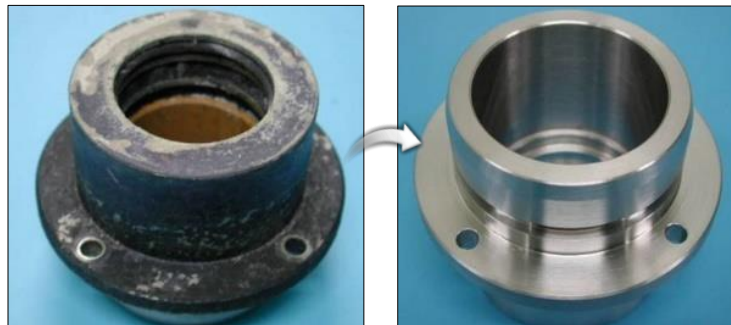
Stainless Steel parts (SUS-304) / Dip 30~60min / @25~50°C
