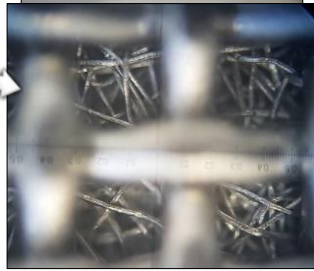
Stainless Steel fiber filter / Dip 60min / @25°C
