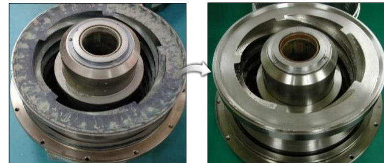
Stainless Steel parts (SUS-304) / Dip 30~60min / @25~50°C
