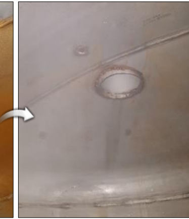
Stainless Steel vessel / Spray 10min / @25°C
