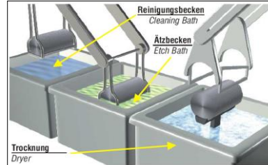
Acid etching(MAE) step (eliminating lapping damages) Remove THK 25~30 \mu m Etch rate : 25 \mu m
